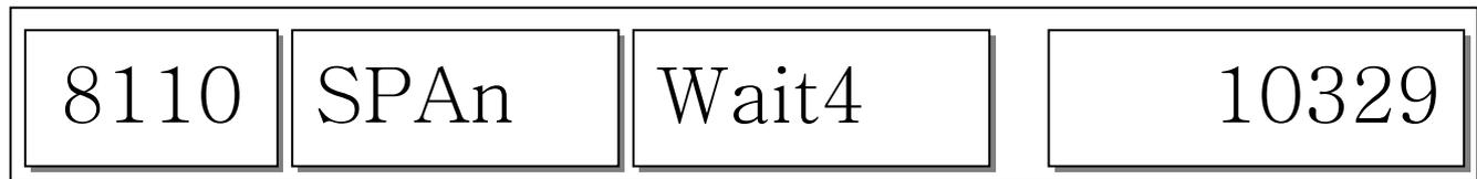
While calibrating zero display shows "Wait4" ~ "Wait0" and follow next message for Span Calibration.
