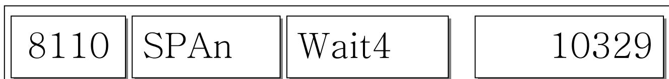
While calibrating zero display shows "Wait4" ~ "Wait0" and follow next message for Span Calibration.
