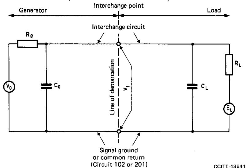
$V_0$  is the open-circuit generator voltage.
