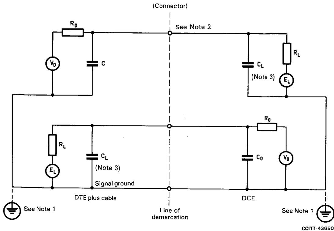
*Note 1* – Signal ground may be further connected to external protective ground if national regulations require.
