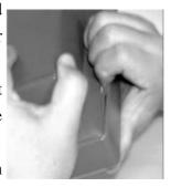
nearest the same corner to release one corner first. Then apply same trick to release the other corner on same side and then the other side to remove the front cover from the back cover. One example of doing so is to follow the alphabetical order (a to h) of the hooks as indicated in the simplified drawing above.
